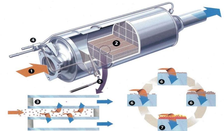
Exhaust gases enter the DPF **1** and pass through the silicon carbide core **2**. The core is designed to have an enormous surface area relative to its compact external dimensions and collects any soot particles present **3**. Pressure **4** and temperature sensors **5** in the DPF casing feed information to the engine ECU, which accurately calculates and monitors the volume of soot held in the DPF to determine the point at which the regeneration should be initiated.
