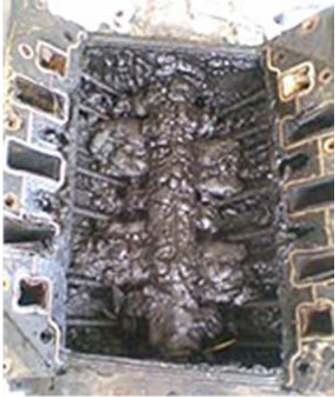
Sludge build up inside a V6 Commodore engine.
